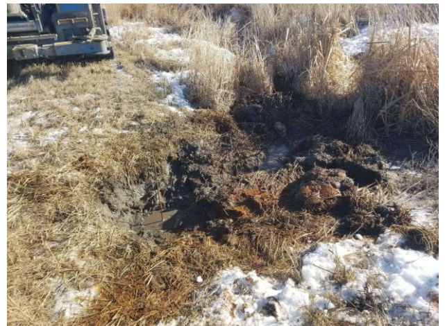
Photo #6 View at borehole 1358-14 (2) – groundwater flowing.
